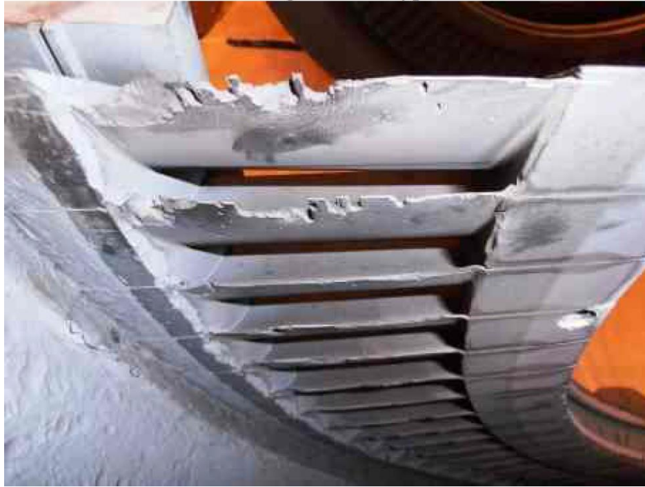
2 Governor UH Blade Ring 1 Row 1 Typical FOD to Blades
